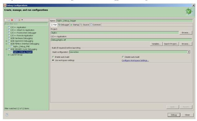
Clicking on **Debug** button the debug will start entering on the first line code of the **main()** function. During the debug session the sleeping mode doesn't work.
